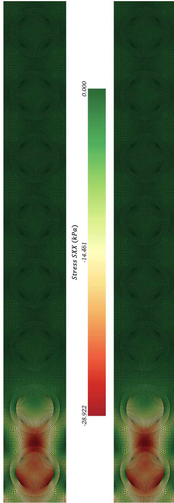
Figure 3.21: Top: Monolithic solution \Omega_{\sigma_{xx}}^{mono} , Bottom: Multi-time step solution \Omega_{\sigma_{xx}}^{mts} ; Elastic wave propagation t = 0.0260 ms.
