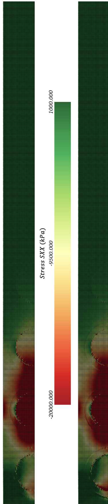
Figure 3.28: Top: Monolithic solution \Omega_{\sigma_{xx}}^{mono} , Bottom: Multi-time step solution \Omega_{\sigma_{xx}}^{mts} ; Elasto-plastic wave propagation at t = 0.0450 ms.
