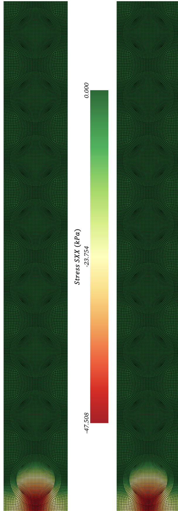
Figure 3.20: Top: Monolithic solution \Omega_{\sigma_{xx}}^{mono} , Bottom: Multi-time step solution \Omega_{\sigma}^{mts} ; Elastic wave propagation at t = 0.0065 ms.
