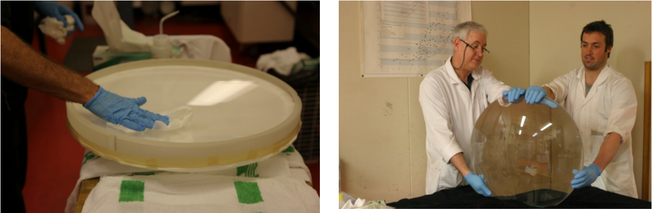
Figure 5: (left) Lens 4 completed. (right) Lens 6 at Kiwistar with the front surface completed, ready to be sent off for aspherisation.
