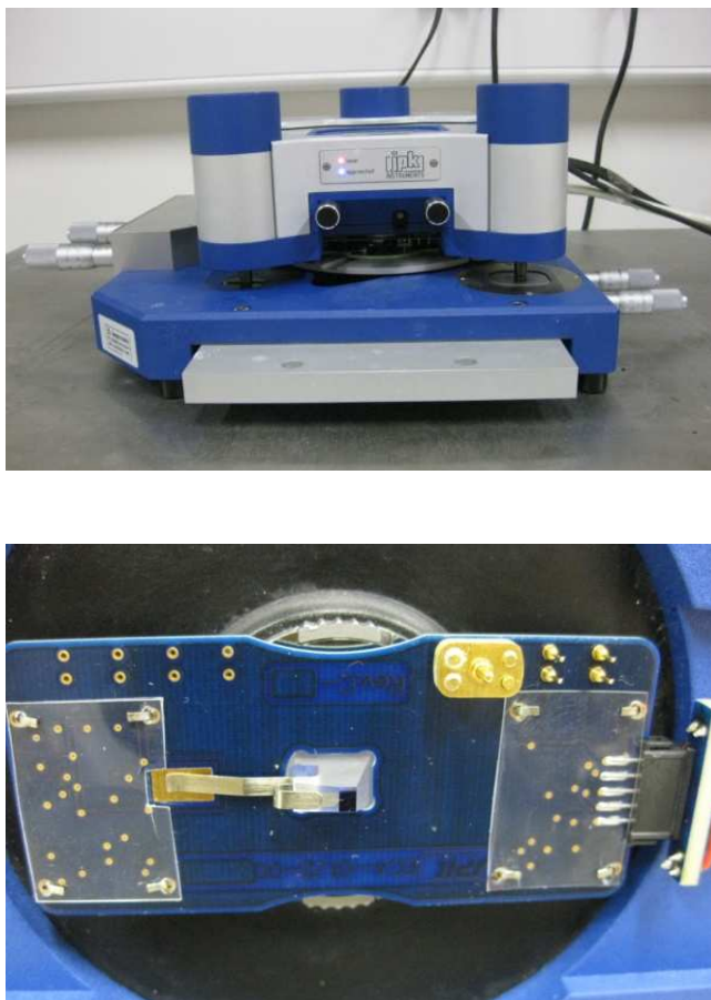
Figure 2.17: The JPK Nanowizard AFM (top) and a magnification of its conducting module (bottom).
