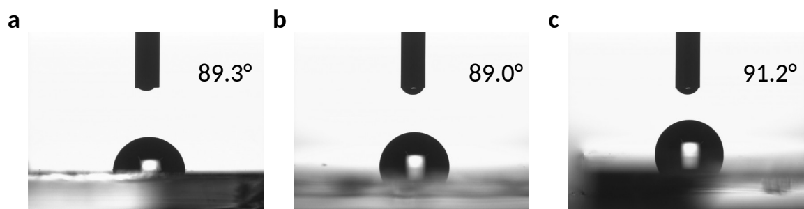
Figure S23. Water contact angles of (a) CB-70 , (b) CD-70 , and (c) CT-70 processed ICBA films fabricated on perovskite layer.
