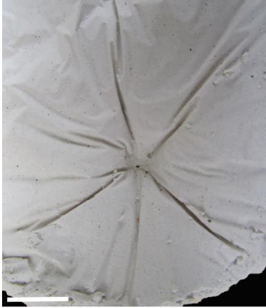
Fig. 1.7. Analogy of the response of mat-bound sediment to fluid pressure, using water injected through sand layer into soft plaster bounded by thin plastic film. Note the development of raised lobes of displaced material between the grooves (cf. lobed discs, Chapter 2). Scale bar: 1 cm.
