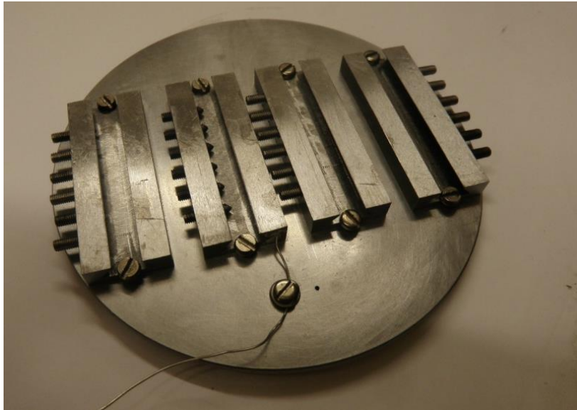
Fig.2.2.1. Implantation plate with thermocouple mounted within the sample holder.
