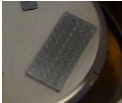
Fig.2.2.2. TEM specimen holder with capacity of holding 46 discs, mounted on the hot stage in the target chamber.
