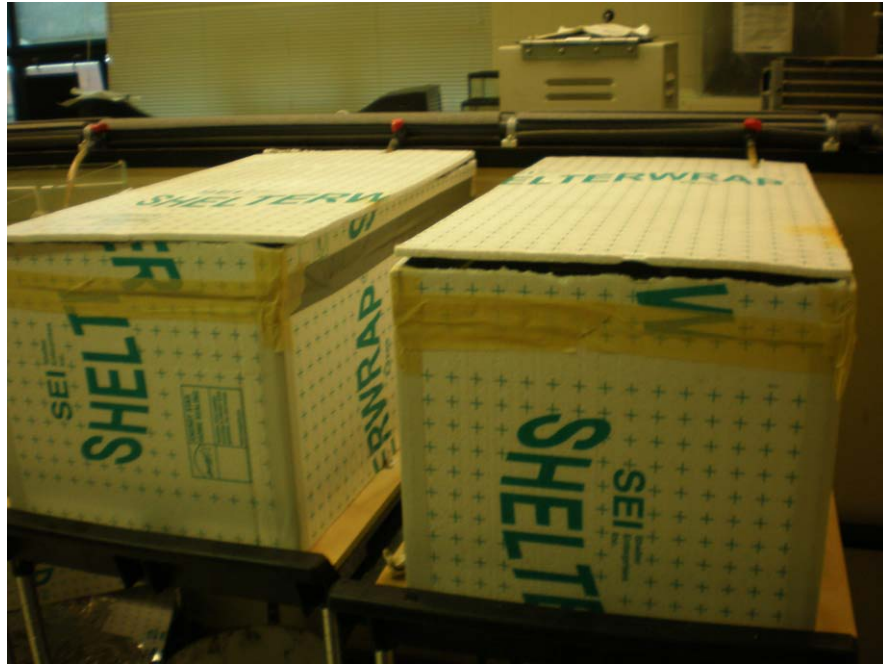
Fig. E1.15. The experimental tanks fully coated with foam to keep out light, therefore preventing photosynthetic micro-organisms from partaking in the degradation of the organic matter. Tank 1 is on the left.
