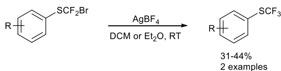
Scheme 4.14 AgBF 4 mediated halogen exchange reaction
