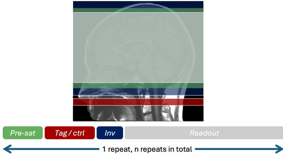
Figure 3.8: Illustration of the CASPRIA sequence, with the spatial locations of each module. The Imaging region and pre-saturation slab cover the whole brain. The single inversion pulse also covers the whole head. The PCASL labeling plane is placed on the neck.
