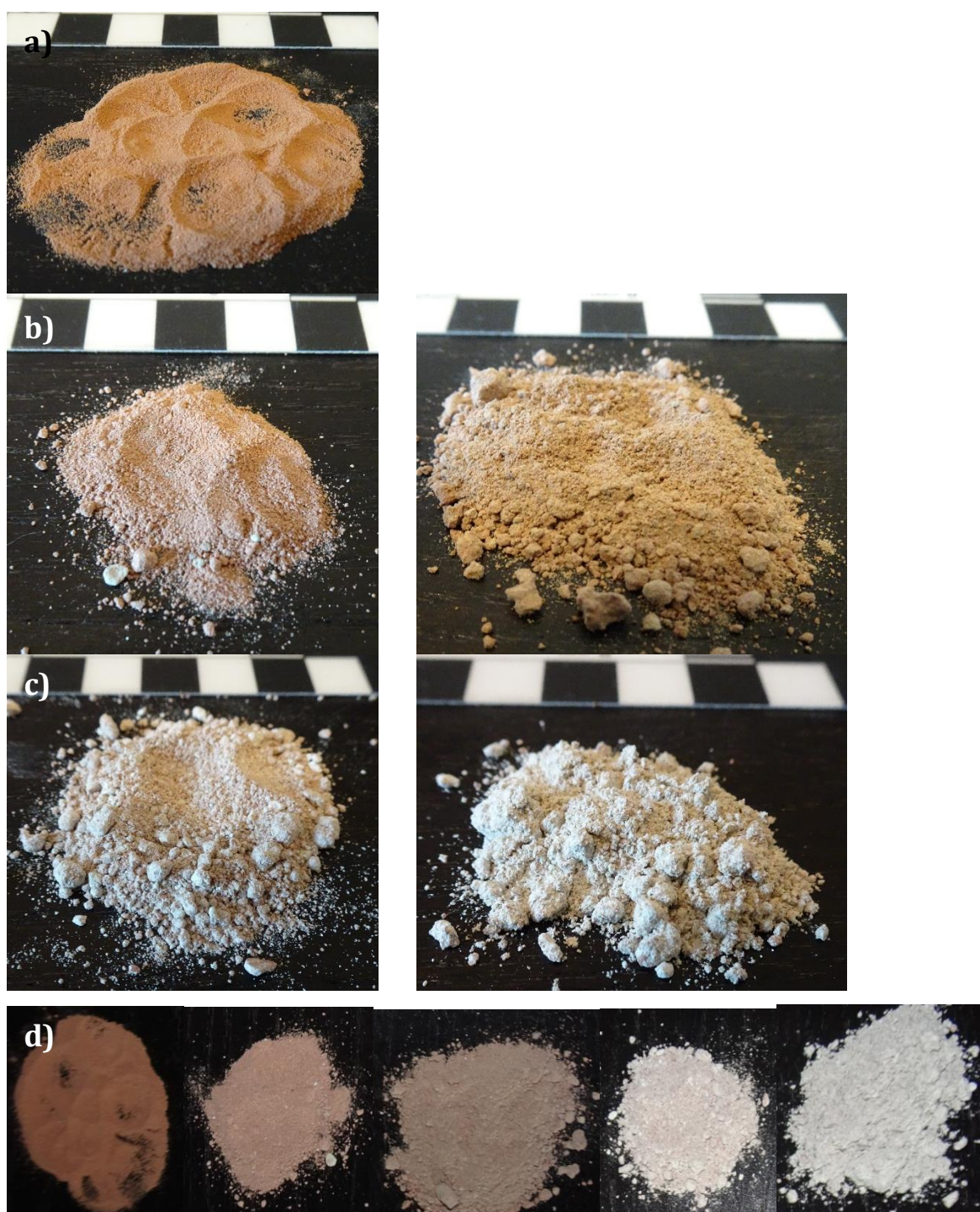
Fig. 6.9. Pulverised fired clay samples due to heavy lime spalling; a) GSC13 900° C b) GSC14, left 900° C, right 1050° C c) GSC16, left 900° C, right 1050° C d) overview of the colour change, from left to right GSC13 900° C, GSC14 900° C, GSC14 1050° C, GSC16 900°, GSC16 1050° C.
