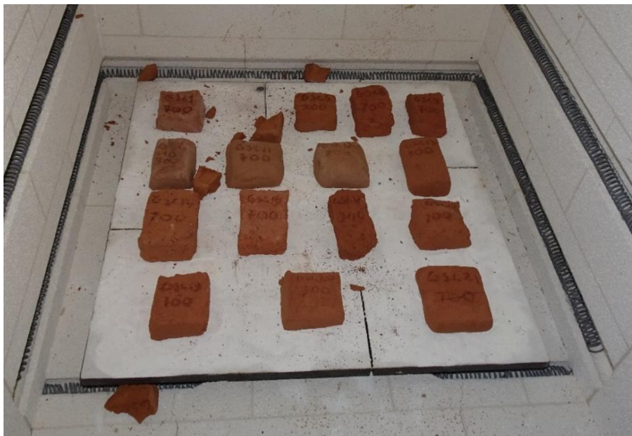
Fig. 4.21. Kiln opening after the first firing; GSC5 exploded into small chunks.
