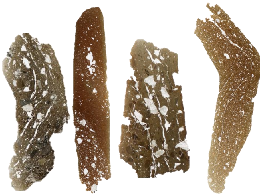
Fig. 5.17. Elongated oblique voids left from coil spreading and joining. Thin section scans, from left to right: CNP13 neck part of a rim sherd, Majiayao; CNP16 body sherd, Majiayao; CNP85 body sherd, Zhujiashai; CNP100 neck part of a rim and handle sherd, Zhujiashai.
