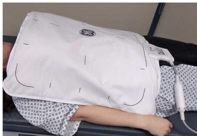
Figure 2.9: Example of an RF receiver coil in position on a participant's abdomen; this is the flexible AIR Coil produced by GE Healthcare, Chicago, USA. Image from Perspectum Ltd.
