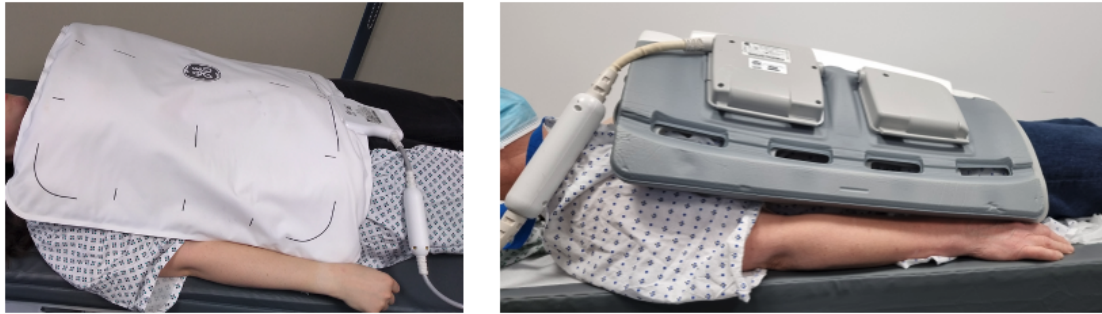
Figure 9.2: Photographs showing two examples of flexible body coils (“flex” coils), which could be used for supine breast imaging as shown here. Images from Perspectum Ltd.
