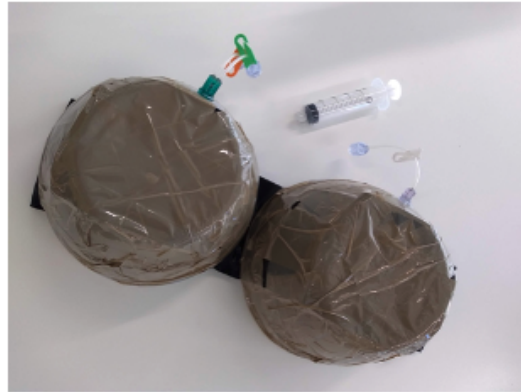
Figure 9.4: Photograph of Prototype 2 of the MR Bra. This support device was made in-house at Perspectum Ltd. from commercially-available plastic cups and included the ability to apply negative pressure. Image from Perspectum Ltd.
