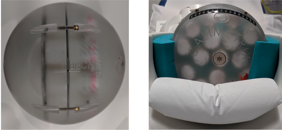
Figure 3.2: Example of a spherical flood phantom, showing the spherical acrylic housing, vials, and LCD thermometer strips. The “CHIN” and “NOSE” markings assist with phantom positioning inside the head coil, shown on the right. Photos reproduced from Perspectum Ltd.
