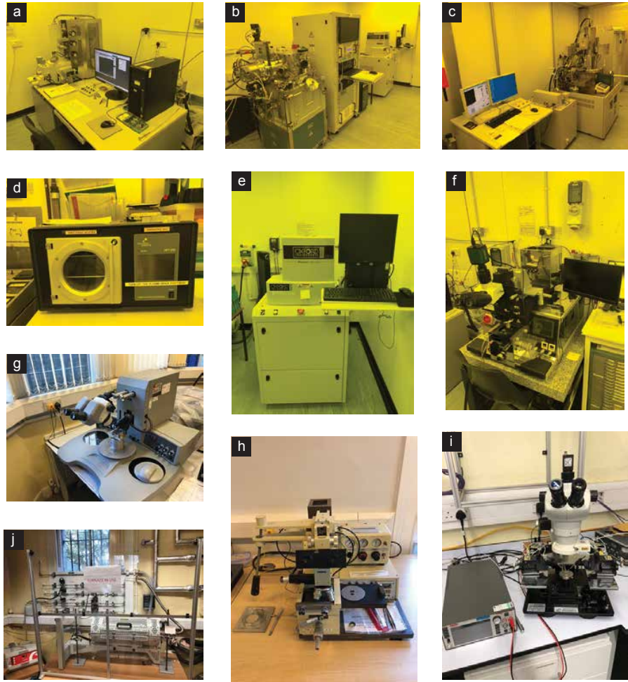
Figure 3.17: Overview of the nanofabrication machines used in this thesis. (a) Hitachi S-4300 microscope. (b) Plassys MEB550S ebeam evaporator. (c) JEOL JBX-5500ZC EBL system. (d) Henniker Plasma HPT-200 plasma treatment system. (e) Oxford Instruments PlasmaPro 80 Cobra ICP RIE. (f) SUSS Mircortech MU84 mask aligner. (g) Kulicke and Soffa Model 4526 wirebonder. (h) Karl Suss mask aligner. (i) Everbeing C Series probe station. (j) Chemical vapor deposition system: Cabolite EVT12300B-23SN tube furnace, equipped with one Alicat MC-2SLPM-D/5M/5IN mass flow controller for argon, and three MC-1SLPM-D/5M/5IN mass flow controllers for hydrogen and methane.
