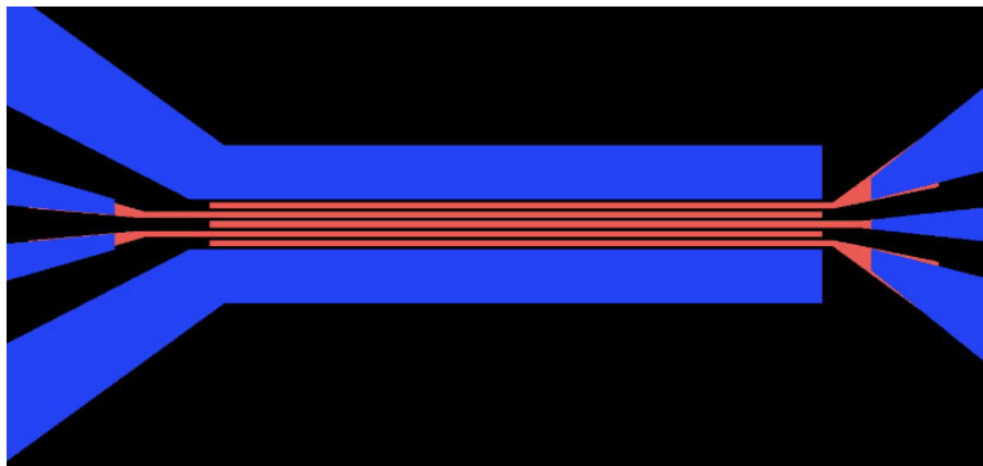
Figure 3.20: Pattern used to expose source, drain and gates during EBL. Source, drain and contact pads are in blue and gates in red.
