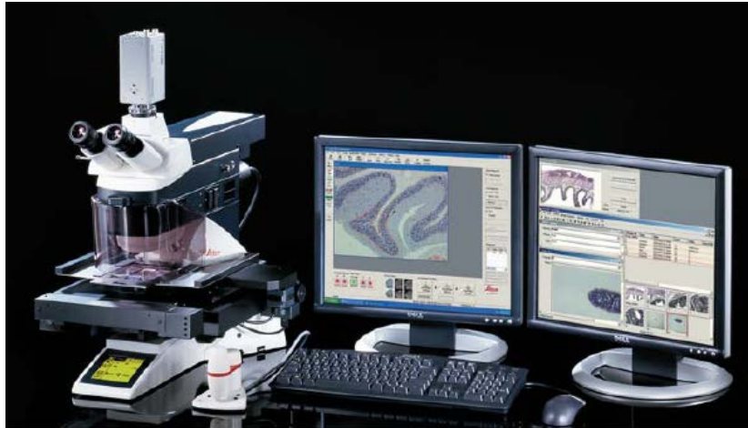
Figure 5-1. A set-up of a typical LCM machine. The image of the section under the microscope is visualised on the computer under a 40X magnification. The cells of interest are manually selected using a drawing tool. The laser, located underneath the slide, cuts out the selected cells and catapults them into a cap of an Eppendorf tube located right above the section.
