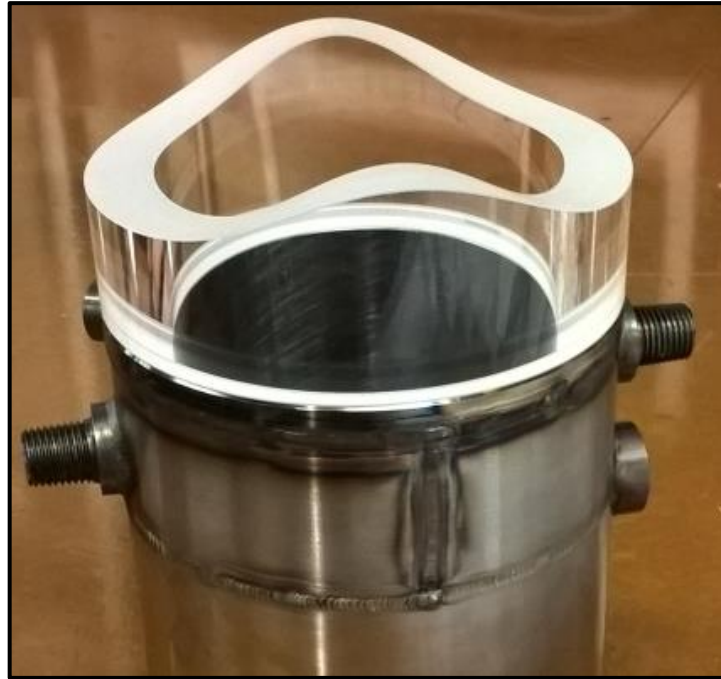
Figure 9-3 New quartz barrel section permitting imaging of the entire pent-roof region from both sides.
