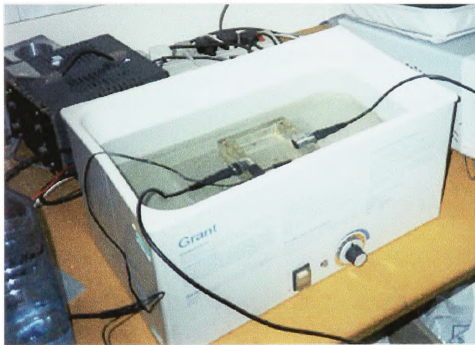
Figure 3.2: Temperature-controlled water bath with Perspex cell inside it.
