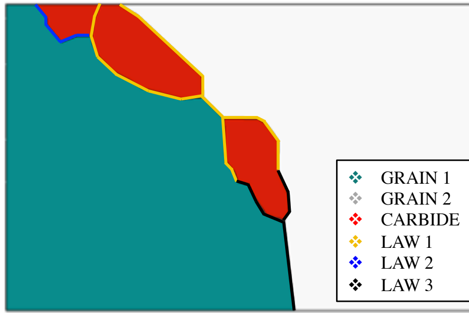
Figure 113: Cut through the center of the cohesive surface FEM model of cantilever R4 before the deformation. The 3 cohesive laws, applied at the individual interfaces, as also summarized in Table 27, are indicated in different colors.
