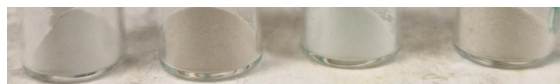
Figure C.28: Photograph of dried Mg_2NiAl LDH catalysts. Left to right: Mg_2NiAl CO_3 , Mg_2NiAl CO_3 AMOST, Mg_2NiAl PO_4 and Mg_2NiAl PO_4 AMOST.
