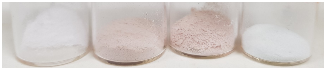
Figure 5.16: Photograph of re-precipitated blends of polypropylene and TM-SLDHs. Left to right: pure PP, PP-Mg 2 Fe SLDH, PP-Mg 2 Fe 0.5 Al 0.5 SLDH and PP-Mg 2 NiAl SLDH.
