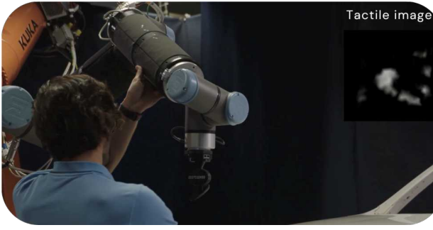
Fig. 4. A physical human–robot interaction scenario with tactile gesture recognition. Both robot links are equipped with ProxySKIN technology.
