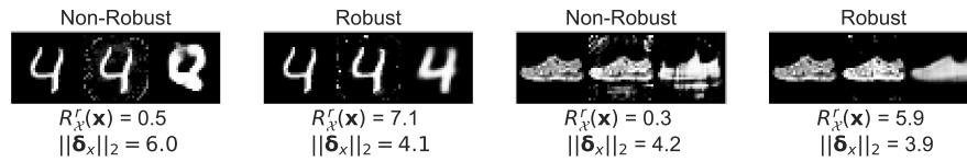
Figure 6.1: Reconstructions under attack for robust and non-robust VAEs. Each subfigure shows from left to right: the original input, a perturbed input made by an adversarial attack, and the reconstruction of the perturbed input. We show results for VAEs that are robust ( R_{\chi}^r(\mathbf{x}) \geq \|\delta_x\|_2 ) and non-robust ( R_{\chi}^r(\mathbf{x}) < \|\delta_x\|_2 ) for a given point \mathbf{x} and adversarially selected perturbation \delta_x . We see that the robust VAE reconstructions are visually closer to the original input.
