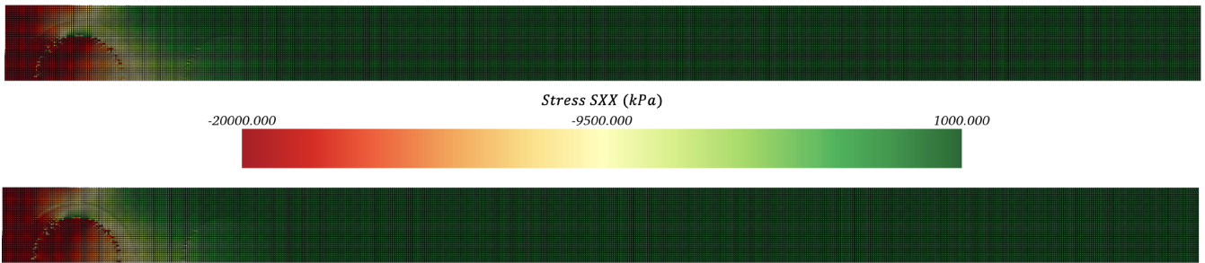
FIGURE 24 | Top: Monolithic solution \Omega_{\sigma_{xx}}^{\text{mono}} , Bottom: Multi-time step solution \Omega_{\sigma_{xx}}^{\text{mts}} ; Elasto-plastic wave propagation at t = 0.015 ms.
