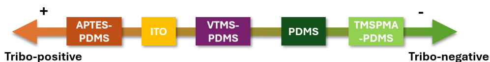
Figure 7.3. Triboelectric series summarising the relative triboelectric properties of the functionalised PDMS and ITO electrode.
