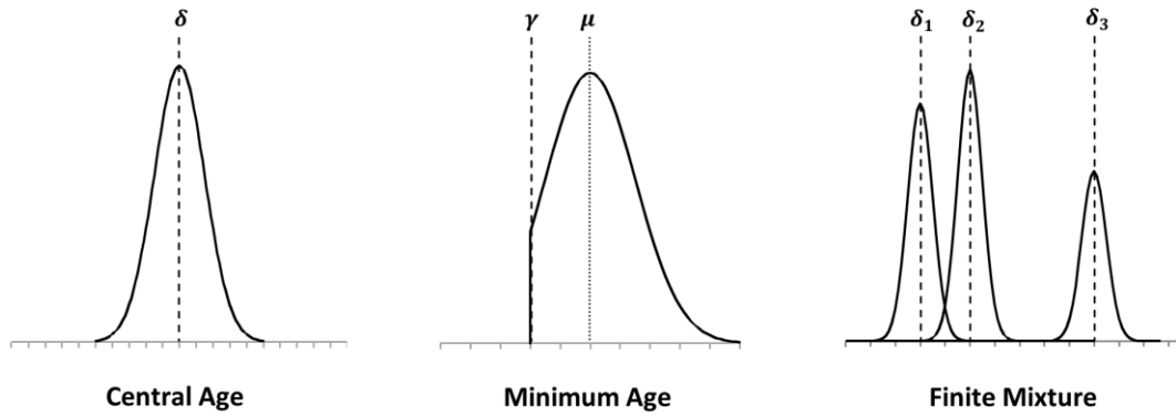
FIG. 4-7. Assumed equivalent dose populations for central age, minimum age, and finite mixture models. The desired equivalent dose is given by either \delta or \gamma . See text for further details.
