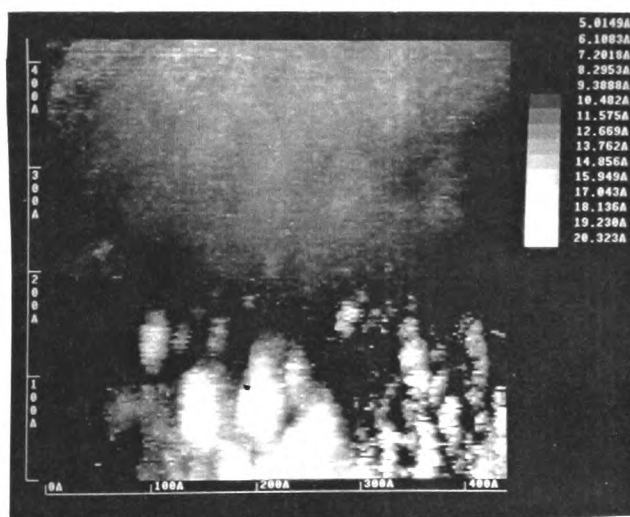
Fig. 6.21. Possible adsorbate effects, sample as for fig. 6.19. t : 1.5 ms, inc : 2.5\text{\AA} , I_T : 2 nA, V_T : 50 mV.
