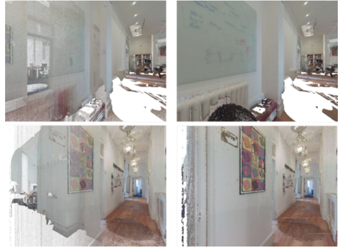
Fig. 4: Images from the left and right sides illustrate the before and after of rendered images from the point cloud when utilizing an adjustable point size based on the distance to the virtual camera.
