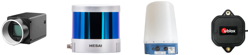
Figure 3.1: From the left to right: Sony IMX camera, Hesai lidar, Navtech radar and Ublox GPS.
