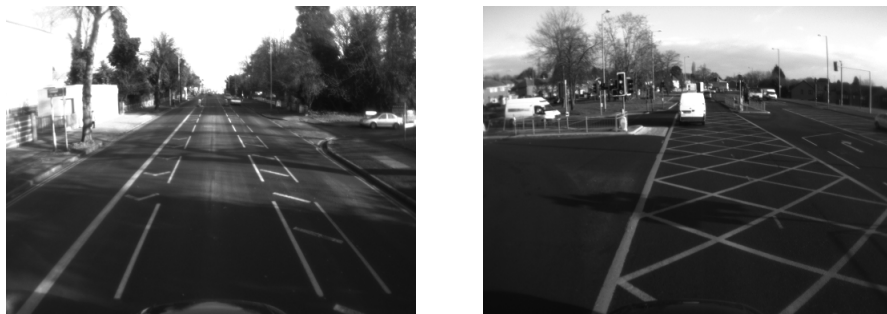
Figure 3.16: The two types of road markings we class as “boxed junctions”. These describe areas of the road that a vehicle should not be stationary in (but possibly quickly traverse) such as separator boxed junctions (left) and intersection boxed junctions (right).
