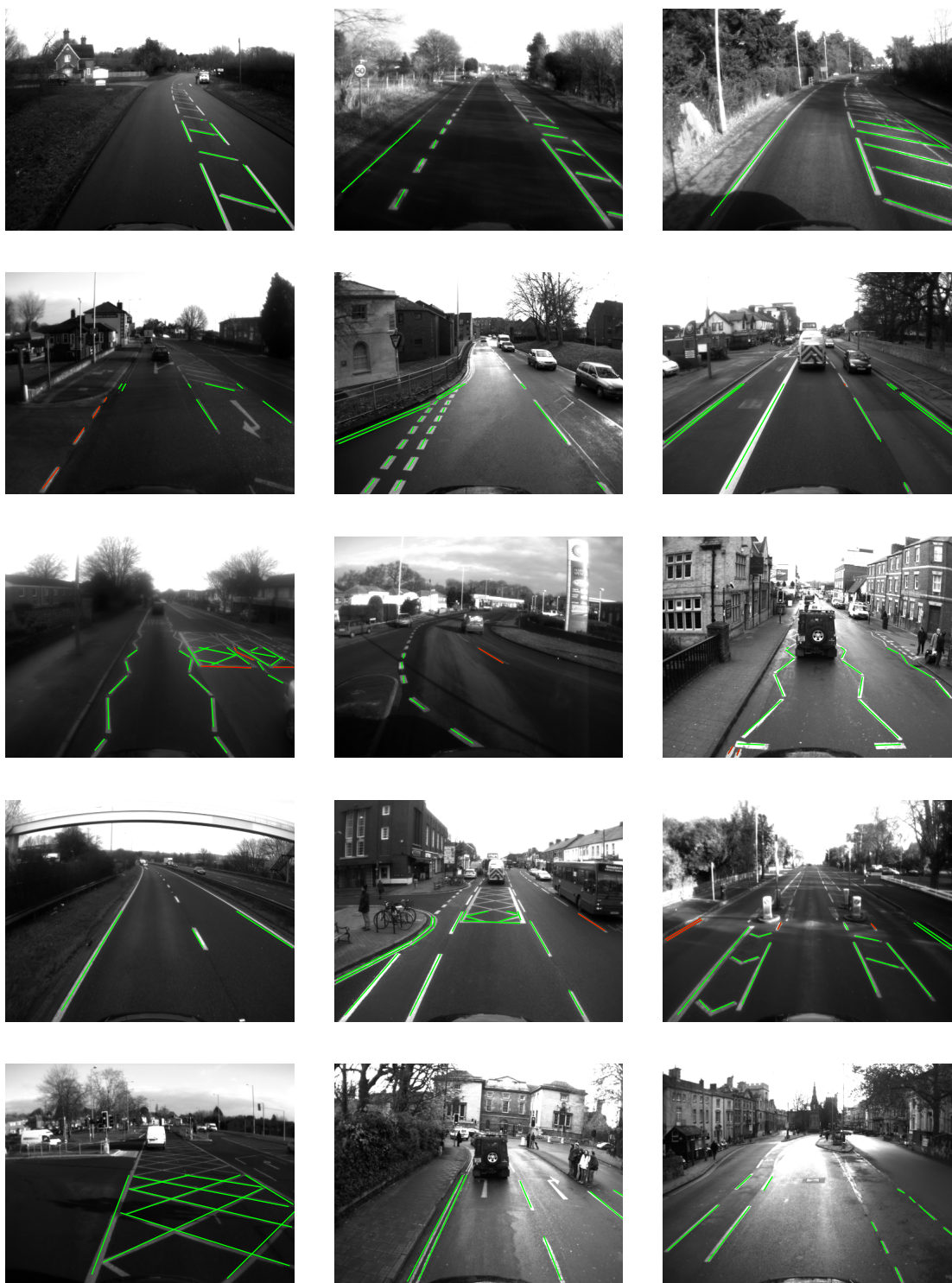
Figure 3.14: Classification results from our system (green lines are correctly classified, whilst red lines represent misclassifications). These images correspond to Figure 3.13.
