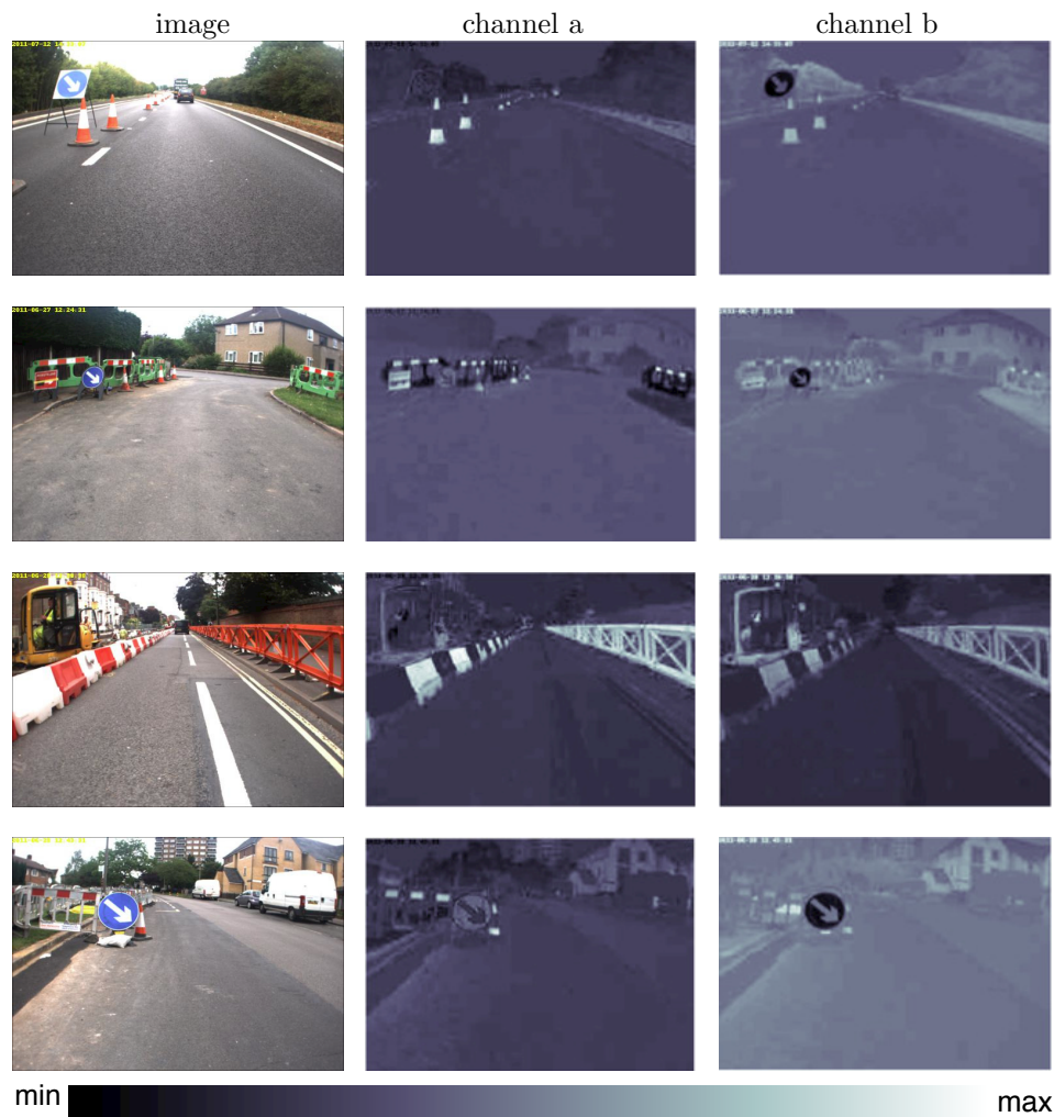
Figure 5.12: Results from our opponent colour spatial prior showing the automatic labelling of pixels in CIE Lab channels a and b. The intensity scale is shown at the bottom of the figure. Notice how blue traffic signs, and barriers/traffic cones are well segmented in channels b and a respectively.
