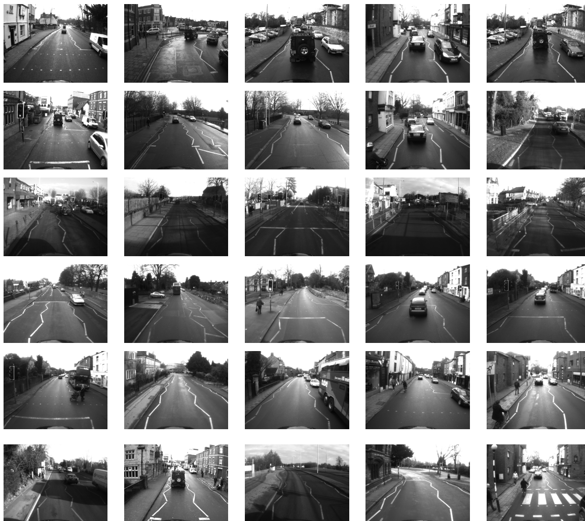
Figure 3.15: Examples of zig-zag approaches correctly classified by our algorithm. Our classification framework achieves a prediction accuracy of 88% for identifying zig-zag approaches and hence anticipating upcoming traffic light controlled pedestrian crossings.
