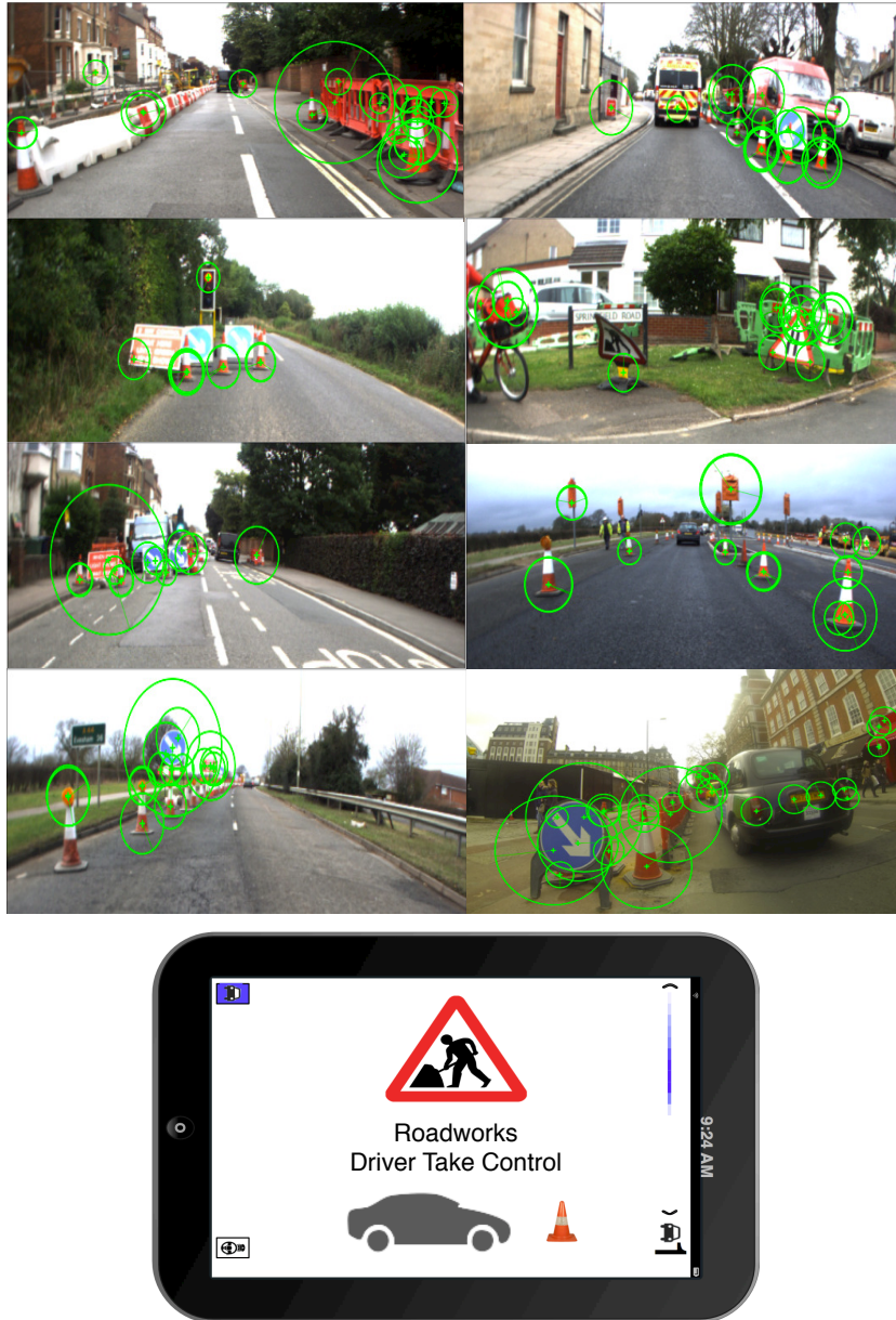
Figure 5.4: Our proposed autonomous vehicle interface for situational awareness at roadwork sites: when roadworks are detected (top), manual control is offered to the driver (bottom). The roadworks shown here were successfully recognised using our roadwork scene signature.
