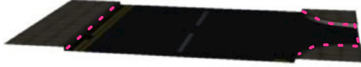
Figure 4.17: A 3D model of a road with and without curbs with road boundary points superimposed in pink. Model taken from Google Sketchup (Trimble 3D Warehouse)[145]
