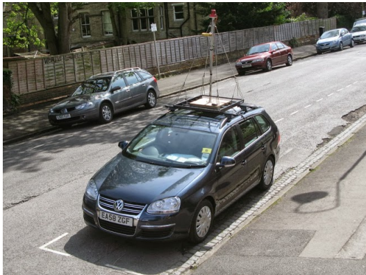
Figure 3.8: Data collection vehicle: the vehicle is shown with a camera rig mounted on the roof [24].
