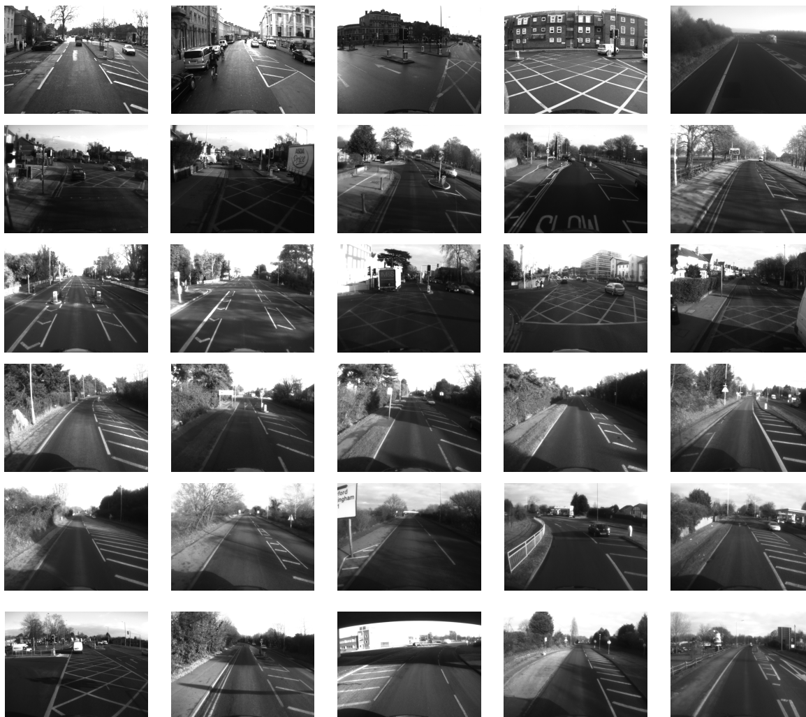
Figure 3.17: Examples of boxed junctions correctly classified by our algorithm. Our classification framework achieves a prediction accuracy of 86% for identifying boxed junctions and hence finding areas of the road where no stopping or traversal is allowed.
