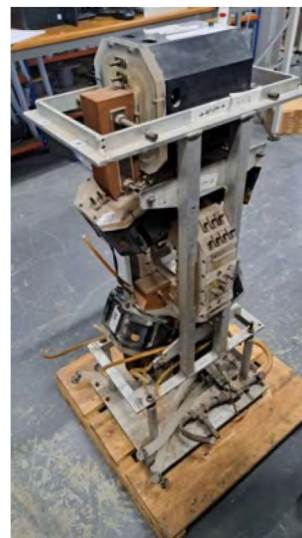
Fig. 1 The current Oxford MSBS with cooling system tubing removed.
