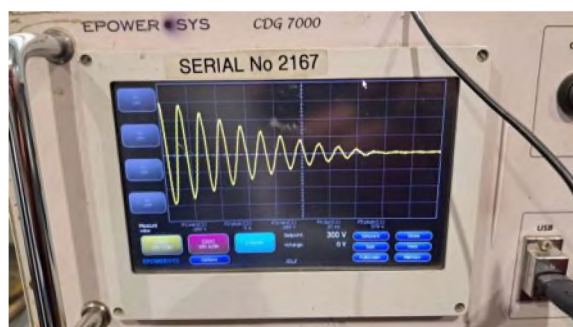
Fig. 5 Pulse test of a pitch coil, showing a good result.
