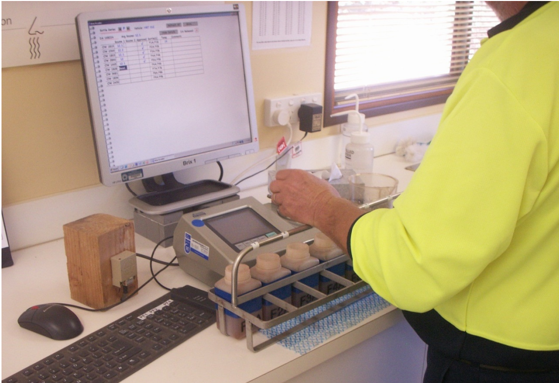
Figure 12: A technician tests the sugar content of freshly-collected juice samples and enters the results into a computer connected to The Company's network.
