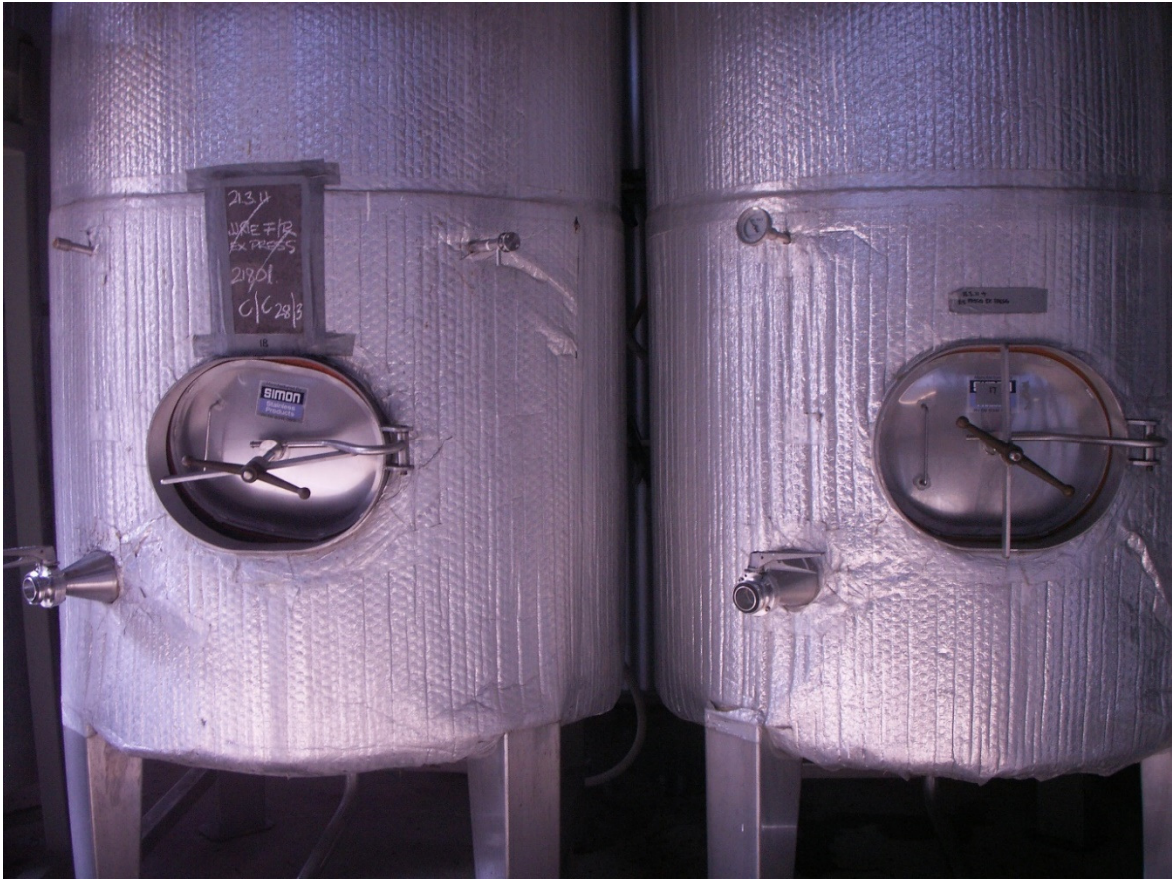
Figure 28: Two fermentation tanks within the Bartoli winery, both of which are labelled as containing free-run Riesling juice.
