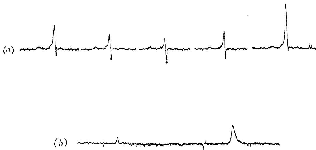
FIGURE 6. (a) Shape of nuclear resonance near zero nuclear polarization for different matching between cavity and waveguide. (b) Nuclear resonance with correct matching.
