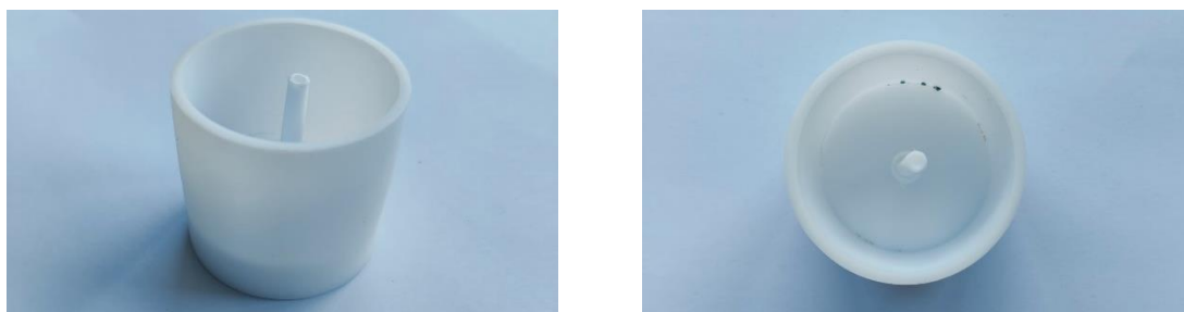
Figure 3.8 HF drip-cup to catch any condensation from the gas inlet, preventing it from hitting the Si surface.
