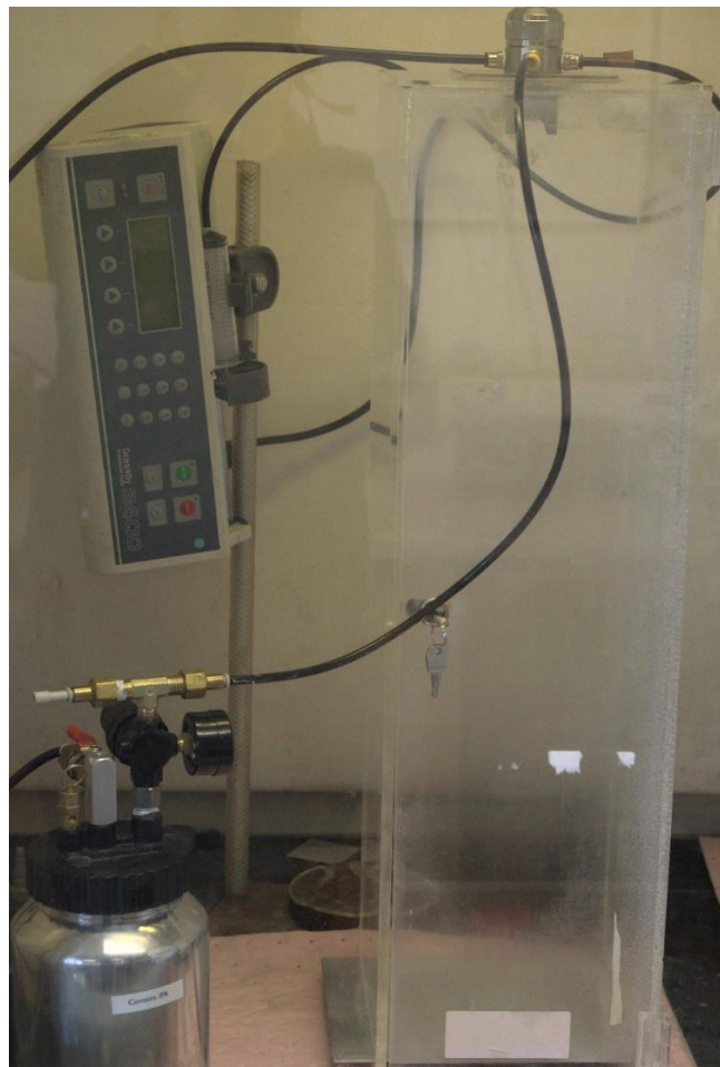
Figure 5.8a) A schematic of the optimised spray unit, including increased box height, IPA reservoir in the atomiser line, and the Al-plate to conceal and reveal wafers to the spray cloud b) a camera image of the optimised spray unit.
