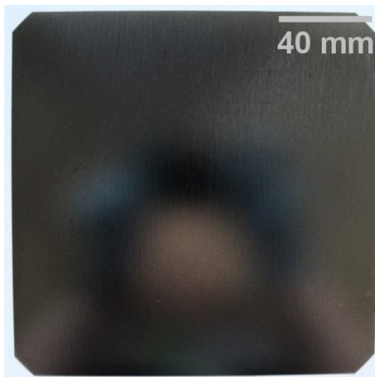
Figure 5.10 Post-texture appearance of three sequentially textured wafers that lost reproducibility.
