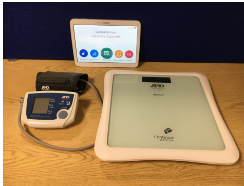
Figure 2.1: Components of the SUPPORT-HF system.
