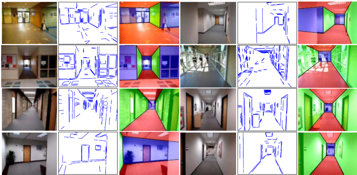
Figure 2.6: Inferred scene structure obtained for single images by Lee et al. [43]. Each triplet shows the original image, the detected line segments, and the final scene geometry. Reprinted with express permission of David Lee.
