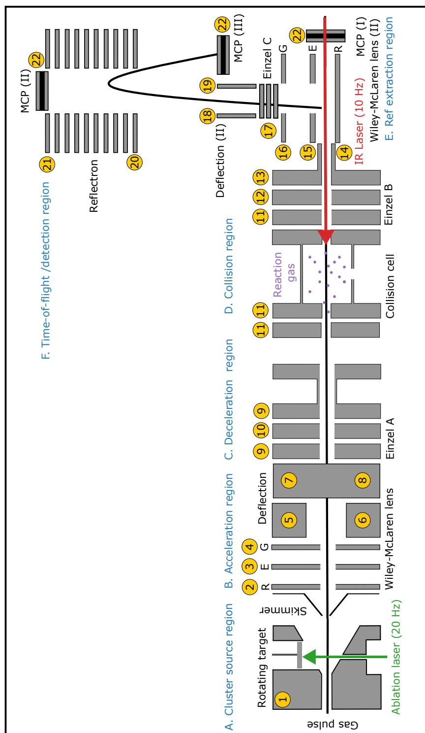
Figure 3.14: Schematic diagram illustrating the components of the linear iteration of the VEC (vibrationally enhanced collision) experiment. The black line illustrates the path of the molecular beam through the experiment. The red and green arrows represent the IR (tunable) and (532 nm) ablation lasers. The yellow circles represent voltages applied to the ion optics/electrodes and correspond to values given in Table 3.3.
