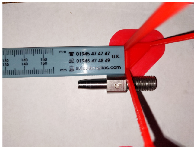
Figure 5.4: An image of a peg that was used in the photographic measurement process. The blue-grey scale can be seen towards the upper portion of the image, and the peg can be seen in the centre of the image. The red additively manufactured alignment jig can also be seen to the right of the image.
