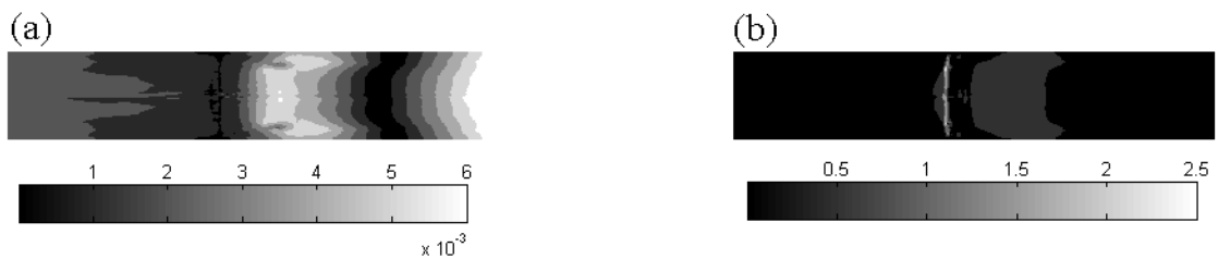
Figure 4.36: 2D lock exchange steady state solution: GCI contours comparing grid configurations \Psi_{8-8} and \Psi_{6-8} at: (a) free surface, and (b) interface.
