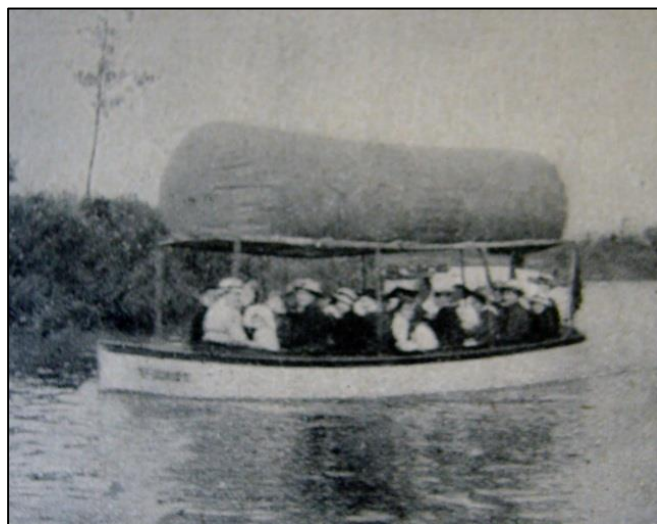
Figure 2.21: Wendy, a craft propelled by coal-gas (1917) 106
