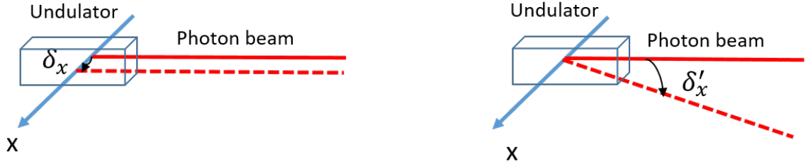
Figure 2.13: Source shift (left) in the horizontal plane with distance \delta_x and tilt (right) in the horizontal plane with angle \delta'_x .
