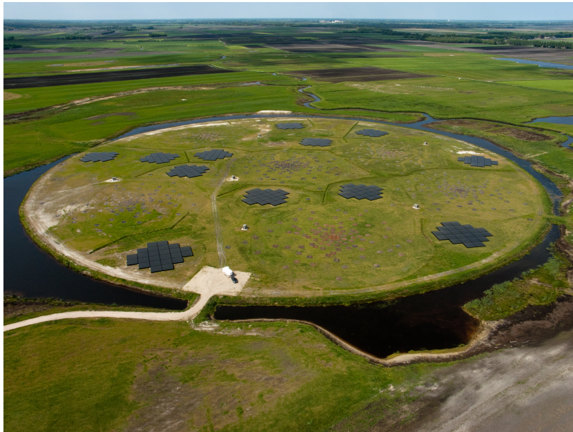
Fig. 2.2 The central part of the core of LOFAR – the so called 'superterp'. It is formed by 6 stations placed on an area of \sim 300 m in diameter, with the remaining 18 core stations arranged across 3 km around it (picture credit: ASTRON)
