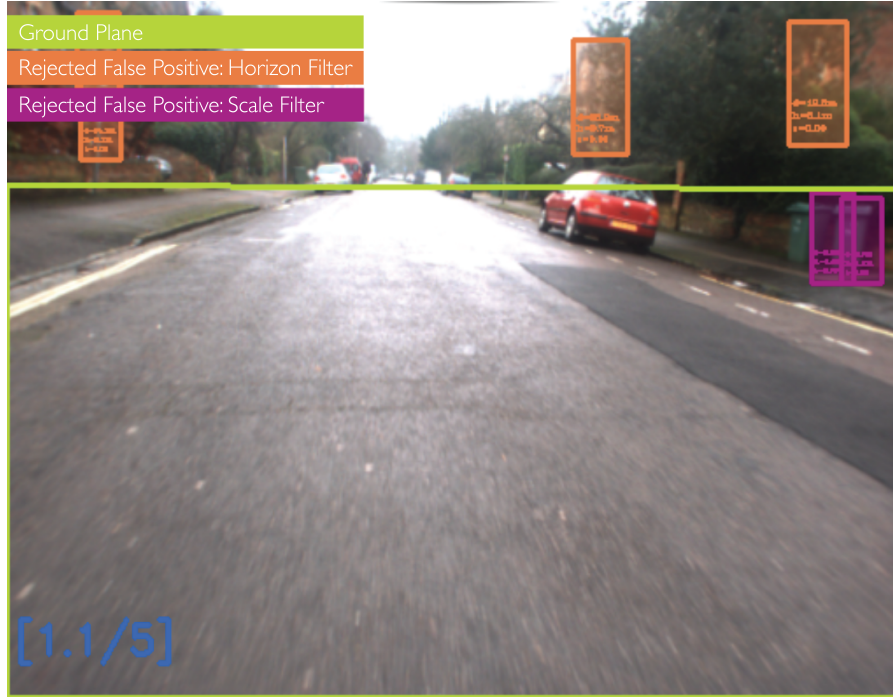
Figure 2.7: Screen capture of the scene filter rejecting candidate detections. Orange boxes are rejected by the horizon filter, whereas purple boxes are rejected by the scale filter.
