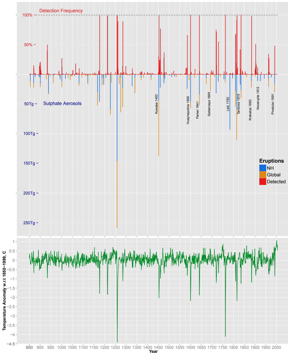
Figure 44: Detected Model Volcanic Eruptions from 850-2005. Top: Detected (red) volcanic eruptions in the model temperature series from 850-2005 using function (a) modelling a single-period drop followed by a reversion to the mean together with an intercept. Bar height indicates detection frequency [0,1] across 100 simulations. Stacked sulphure deposition record used to force model temperatures are shown for Northern hemisphere (blue) and global measurements (orange) in Tg. Bottom: simulated model mean temperature anomalies (green) used to detect the above volcanic eruptions. Mean NH surface temperature data is taken from the Last Millenium and historical simulation of the NCAR CCSM4 model as part of the CMIP5/PMIP3 data archive.
