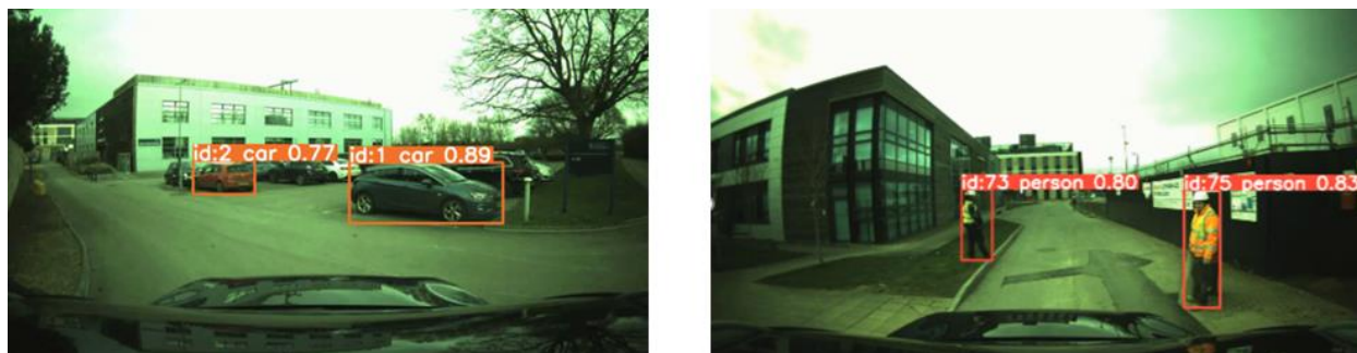
Figure 10. Results of Object Detection. (Left) Detection of vehicles, including classification labels and confidence scores. (Right) Detection of pedestrians.
