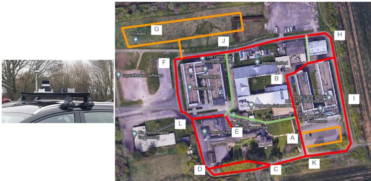
Figure 6. (Left) SafeMove Payload mounted on an electric vehicle using a standard roof rack. (Right) Overview of Oxford's Begbroke Business Park. The red lines represent normal roads, the orange sections indicate car parks, and the green paths correspond to pedestrian paths. Waypoints labeled A through L represent starting and destination points for point-to-point missions. The route spans 800 meters per loop, totaling approximately 2 kilometers.
