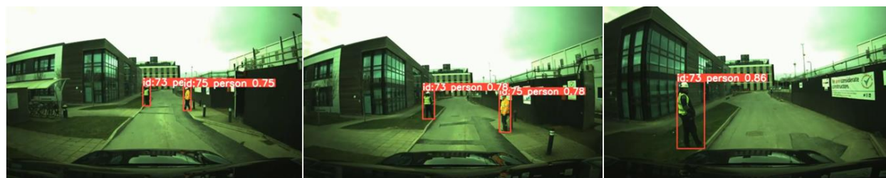
Figure 11. Results of Object Tracking. The sequence demonstrates robust tracking performance, with ID 73 consistently assigned to a person throughout the scenario and ID 75 assigned to another individual for part of the sequence. A video demonstrating these results is available at https://youtu.be/r9t8vxUKLP0
