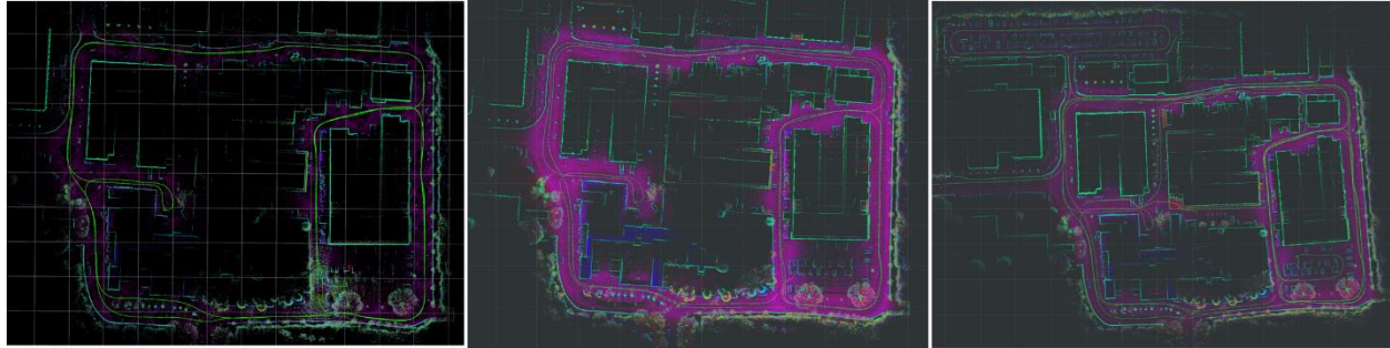
Figure 7. Results of Multi-Sensor Mapping. Left image shows a single-session map, center image demonstrates the combined map after three sessions, and right image presents the extended map after six sessions. This sequence demonstrates the system’s ability to integrate data from multiple mapping sessions, progressively extending the operational area while ensuring detailed and accurate representations.
