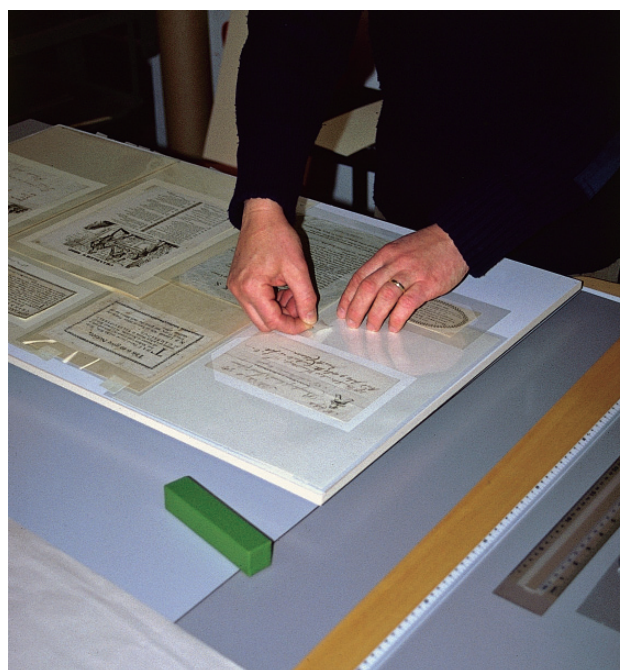
Figure 3 Taping the overlapped polyester slings to a panel.
