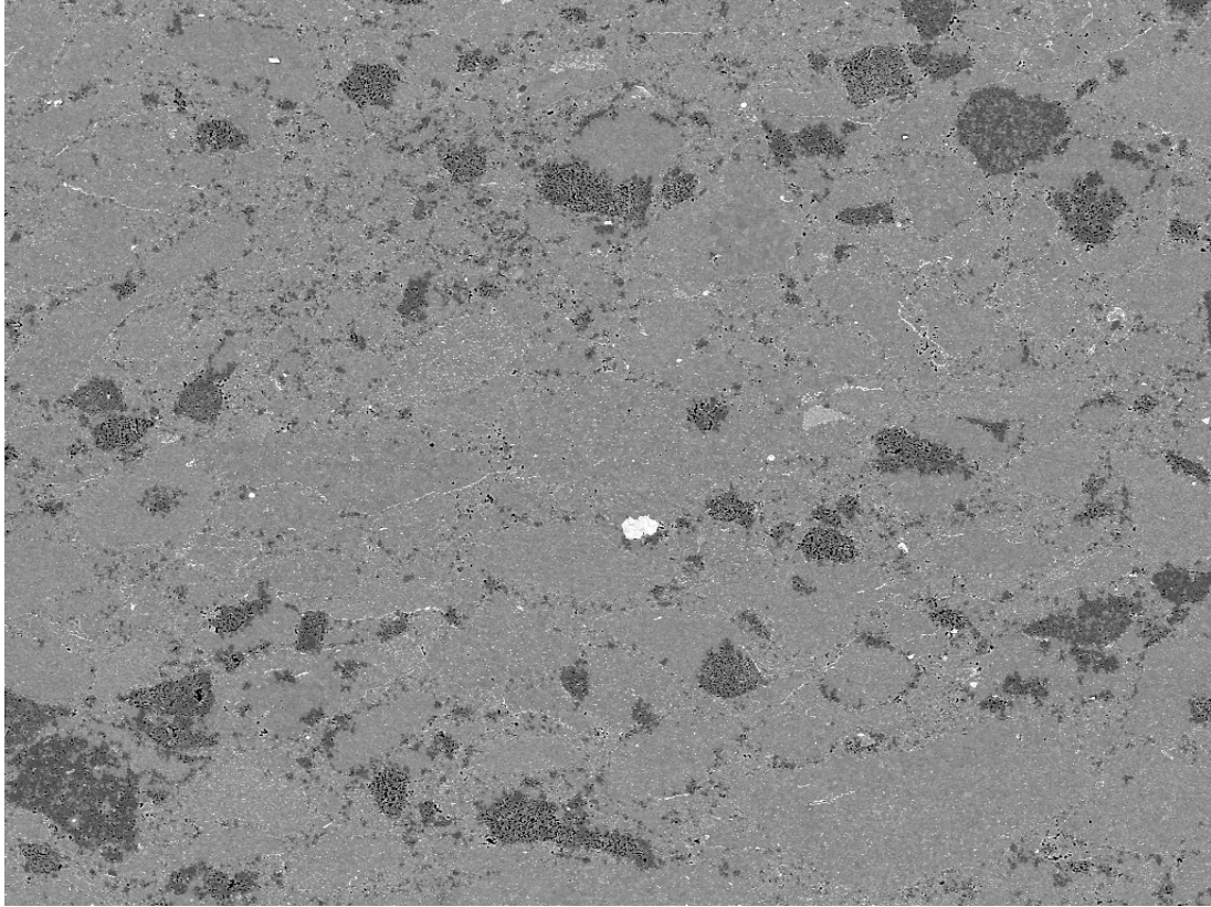
Figure 2.5: Initial backscattered image used for the image processing method (250x magnification).
