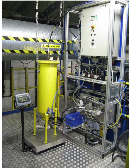
Figure 3.4: DACS co-injection pump and yellow hopper.
