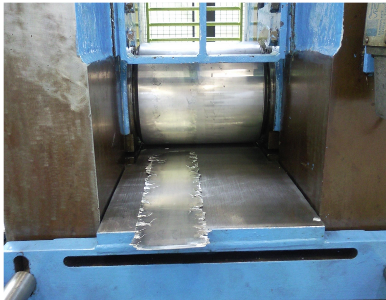
Figure 6.12: The roll mill showing accumulative roll bonding of Al-4Cu+Ti.
