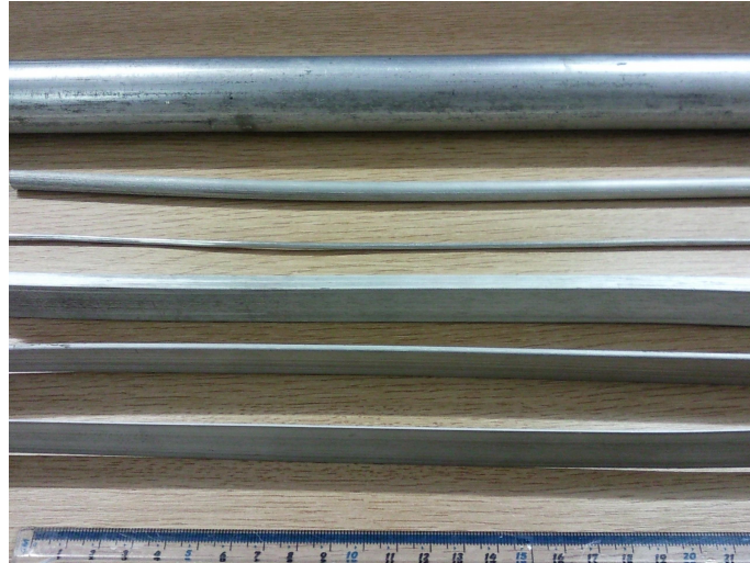
Figure 4.7: Al-12Si+Ti \Phi 30\text{mm} bar that was further extruded to: \Phi 7.5\text{mm} and \Phi 2.5\text{mm} cylindrical bars and 6mm; 2.5mm; and 1mm thick rectangular strips at different deformation ratios.
