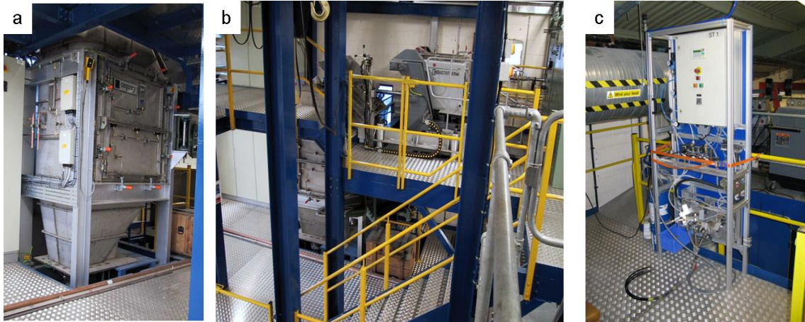
Figure 3.8: The spray forming plant at the Begbroke Science Park, Oxford. The spray forming chamber is shown to the left, the induction furnace is shown in the center and the DACS co-injection powder pump is shown to the right.
