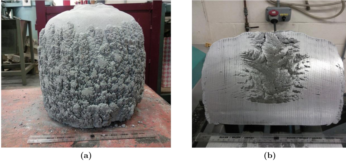
Figure 5.15: (a) Al-4Cu+Ti composite billet processed by spray forming (AlCuTi3) and (b) a cross-section of AlCuTi3 where the region of co-injection is visible throughout most of the billet.
