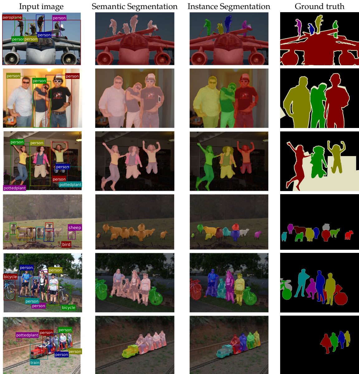
Figure 4.9: Success cases of our method. First and second row: Our algorithm can leverage good initial semantic segmentations, and detections, to produce an instance segmentation. Third row: Notice that we have ignored three false-positive detections. Additionally, the red bounding box does not completely encompass the person, but our algorithm is still able to associate pixels “outside-the-box” with the correct detection (also applies to row 2). Fourth row: Our system is able to deal with the heavily occluded sheep, and ignore the false-positive detection. Fifth row: We have not been able to identify one bicycle on the left since it was not detected, but otherwise have performed well. Sixth row: Although subjective, the train has not been annotated in the dataset, but both our initial semantic segmentation and object detection networks have identified it. Note that the first three images are from the VOC dataset, and the last three from SBD. Annotations in the VOC dataset are more detailed, and also make more use of the grey “ignore” label to indicate uncertain areas in the image. The first column shows the input image, and the results of our object detector which are another input to our network. Best viewed in colour.
