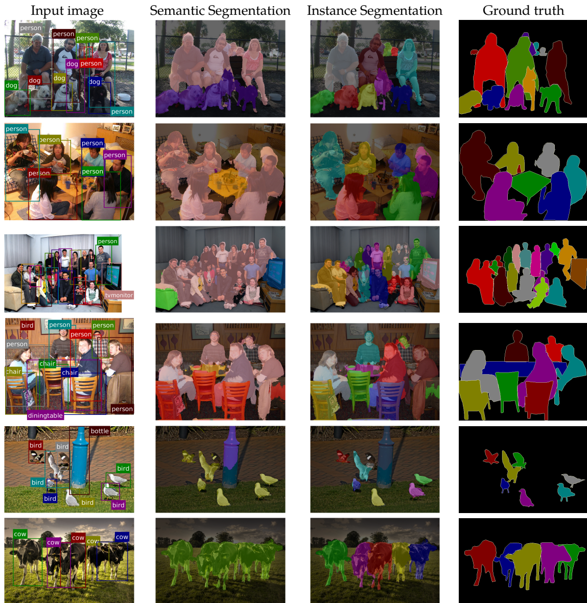
Figure 4.10: Failure cases of our method. First row: Both our initial detector, and semantic segmentation system did not identify a car in the background. Additionally, the “brown” person prediction actually consists of two people that have been merged together. This is because the detector did not find the background person. Second row: Our initial semantic segmentation identified the table, but it is not there in the Instance Segmentation. This is because there was no “table detection” to associate these pixels with. Using heuristics, we could propose additional detections in cases like these. However, we have not done this in our work. Third row: A difficult case where we have segmented most of the people. However, sometimes two people instances are joined together as one person instance. This problem is because we do not have a detection for each person in the image. Fourth row: Due to our initial semantic segmentation, we have not been able to segment the green person and table correctly. Fifth row: We have failed to segment a bird although it was detected. Sixth row: The occluding cows, which all appear similar, pose a challenge, even with our shape priors. The first column shows the input image, and the results of our object detector which are another input to our network. Best viewed in colour.
