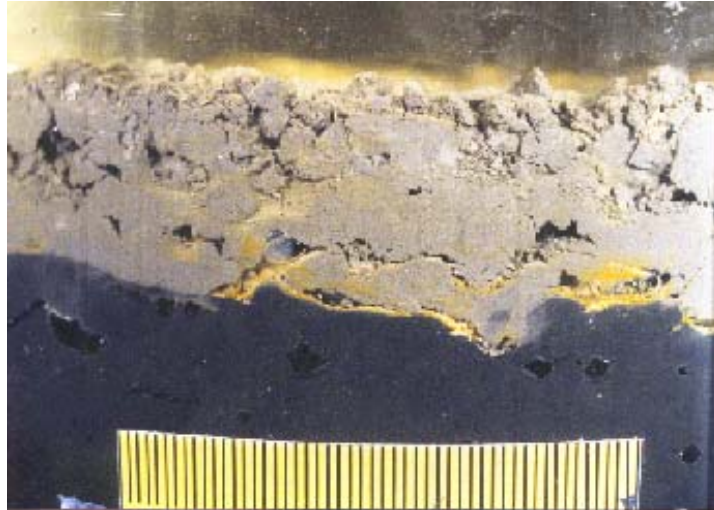
Figure 7.8 Low density layer at the top of a slurry deposited bed is characterised by a different colouration, and often gas bubbles, as seen in this extreme case. Photo courtesy of Ramon Gonzales, Department of Engineering Science, Oxford.
