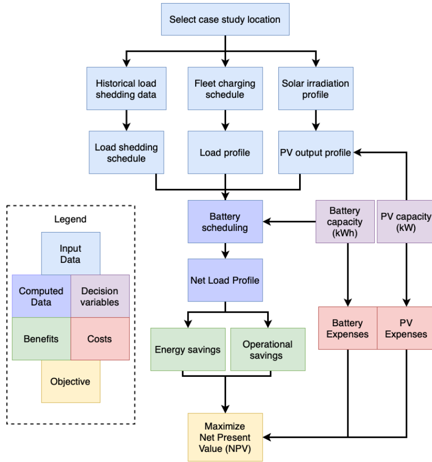
Figure 6.1: Flow chart of optimization model to determine the PV and battery sizes that maximize net present value.
