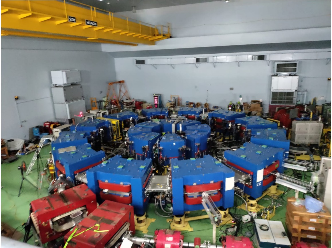
Figure 4.2: Photograph of the KURNS main ring FFA [76]. This displays the return-yoke-free magnet design, where the gap of the F-magnet can be seen and accessed from the outer and inner sides of the magnets. The extraction line is visible towards the left-hand side of the picture, where it can be seen exiting the azimuthal centre of one of the F-magnets. The central smaller ring is the BOOSTER ring, which was originally used as part of the injection system, but is no longer operated.
