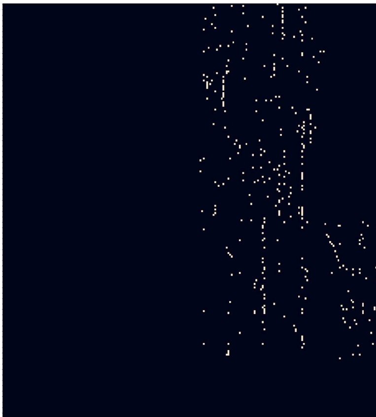
Fig 2. Adjacency matrix of the supply chain network plotted as a “seaborn” heatmap: each node has a position along x and y axis, White dots indicate links (1’s) from x-node to y-node. Large black area on the left corresponds to zero in-degree for the pharmacies and OTCs (low node index), black area top right indicates no links from suppliers to retailers, and the black area at the bottom indicates no known out-degree for the top level suppliers.
