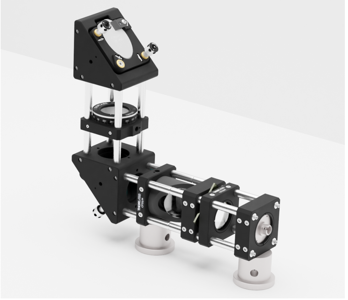
Figure 8.2: 3D render of the MOT periscope for one of the four horizontally propagating beams. Light from an optical fibre is collimated by an achromatic lens. The light passes through a voltage-controlled LCD variable retarder, which rotates the polarisation of the light before it is passed through a linear polarising plate. This allows a controllable amount of power after the linear polariser. A 10:90 beam sampler splits off light to be measured by a photodiode, which provides an error signal to actively stabilise the beam power using the LCD waveplate. Light is then steered with two right-angled elliptical mirrors to elevate the beam to the height of the glass cell and passes through a circular polariser to obtain the correct \sigma polarisation for the cooling transition. Model provided by Abel Beregi.
