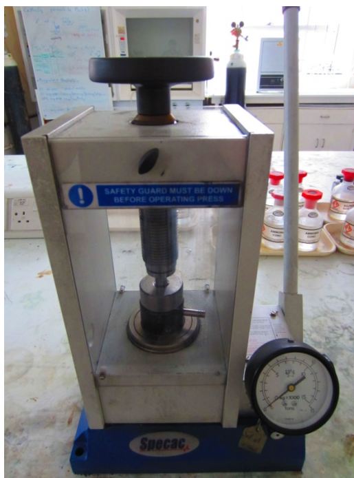
Figure 3.1. The photograph of a hydraulic press and a pellet die for the construction of 3D porous carbon electrodes.
